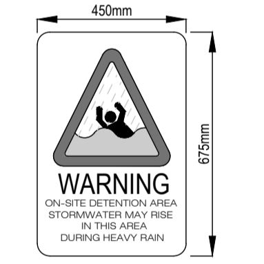
ON-SITE DETENTION WARNING SIGN NTS
