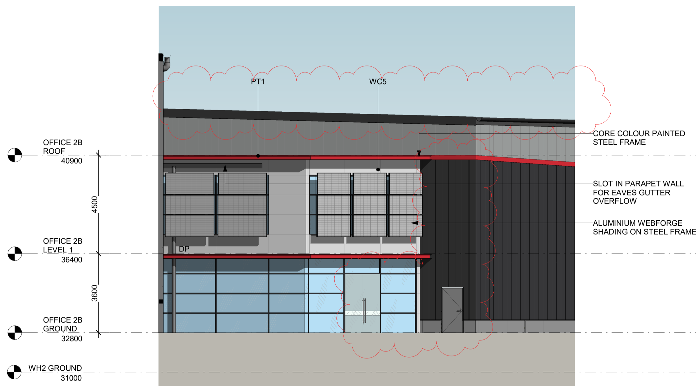
1 OFFICE 2B EAST ELEVATION A112 1 : 100
