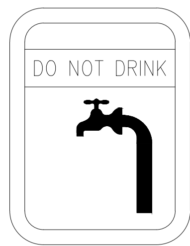
DETAIL 1 RAINWATER SIGN SCALE 1:10
