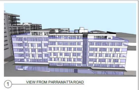
Figure 11: Height plane diagram showing the building elements that exceed the height limit
