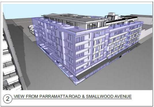
Figure 12: Height plane diagram showing the building elements that exceed the height limit
