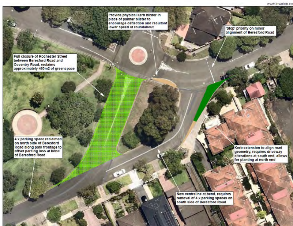
Figure 1. Schematic of closure of Rochester Street through Davey Reserve.
