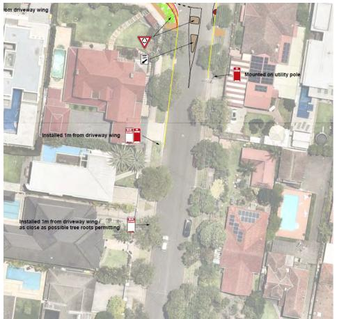
Figure 6 – signage plan for the relocated bus stop
