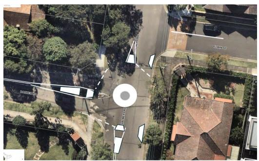
Figure 1 – preliminary concept design of roundabout at the intersection of Barker Road and Chalmers Road
