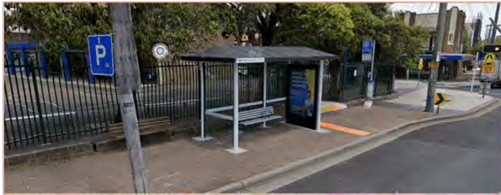
Figure 49: Bus Stop Footpath Pinch Point
