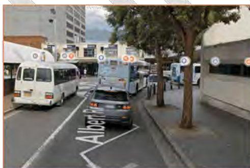
A vehicle approaching the 90-degree turn is unsighted to the zebra crossing 35 metres downstream
