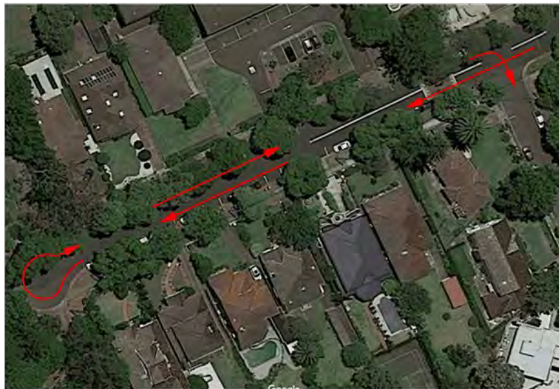
Figure 4 – traffic manoeuvres to allow residents to turn right into Allenby Crescent during the hours of effect of the proposed left turn restriction
