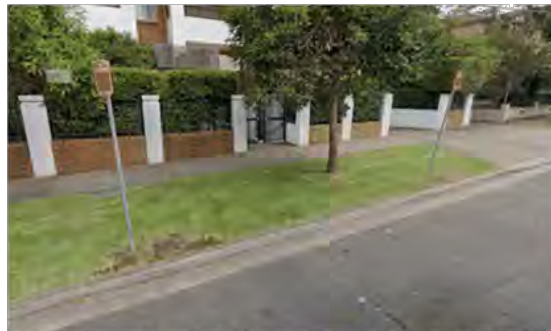
Figure 1 – 'No Stopping' signs within 7m of each other not needed due to perception of sign defining the zone
