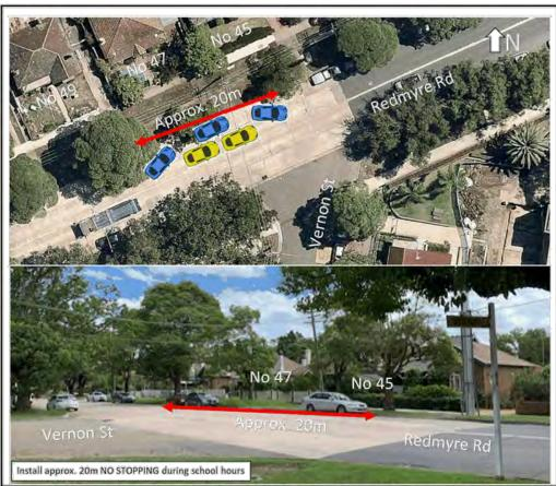
Figure 1 - VERNON - Proposed parking changes at the intersection of Redmyre Road and Vernon Street
