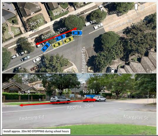
Figure 2 – MARGARET – Proposed parking changes at the intersection of Redmyre Road and Margaret Street
