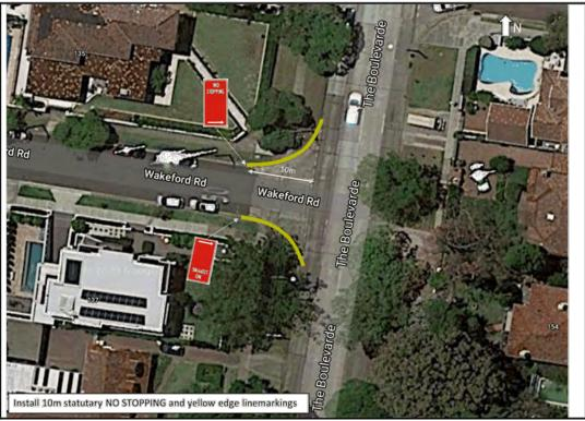
Figure - Plan of 10m Statutory NO STOPPING and yellow edge linemarking in Wakeford Road
