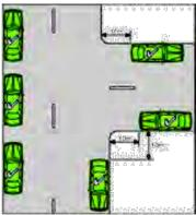
Figure – Example Measurement of distance at t-intersection without traffic lights (Source: NSW Road Rules 2014)
