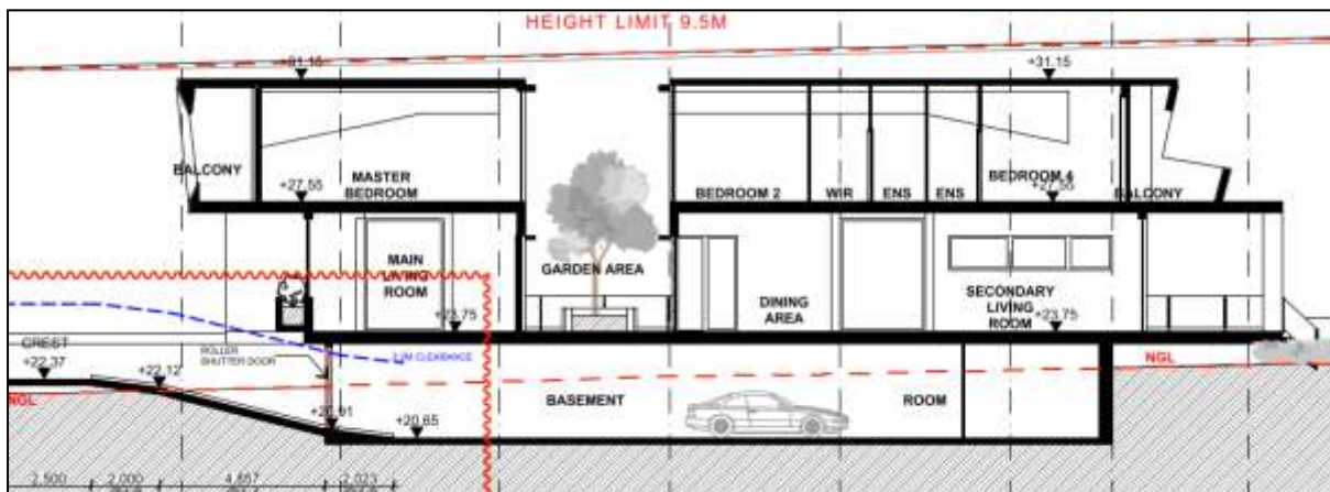
Figure 21: Original Section Plan. Note raised height of finished floor level above natural ground and overall building heights including excessive floor to ceiling heights.
