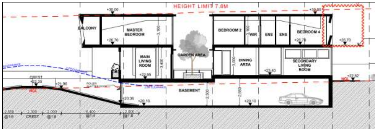
Figure 22: Revised Section plan showing a compliant basement height, compliant floor to ceiling heights and overall reduced building height.
