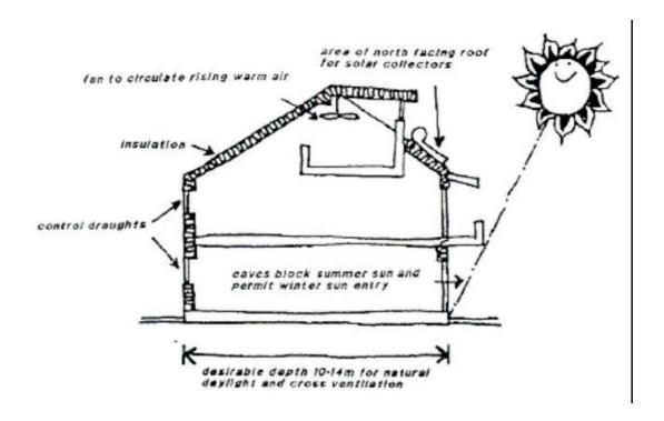
Figure 3 – Buildings designed to maximise benefits of energy efficiency Source: Urban Form, Urban Design & Energy Use: Occasional Paper Series 2 Paper 2
