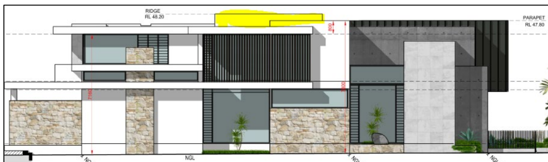
Figure 11: Proposed (west) side elevation with non-compliant raised element highlighted in yellow.
