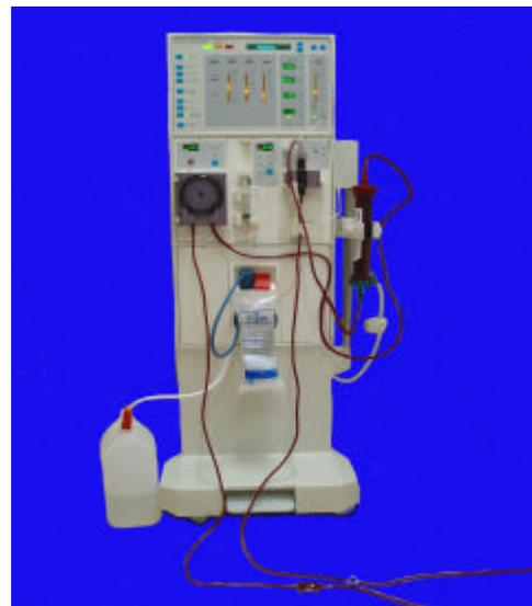
One type of machine used for home haemodialysis showing liquid concentrate container, bi-carb bag (centre), bloodlines, and dialyser (at right).
